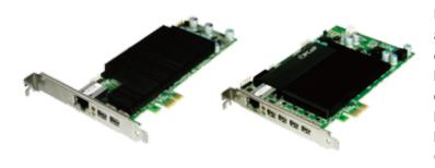
PCoIP remote acceleration cards can be added to any existing PC or workstation to enable field-proven high-end 1:1 session leveraging PCoIP protocol graphics and desktop performance. It's the only hardware remote solution which can allows high-end 3D applications with dedicated GPUs that is not available when using virtualized desktops.
